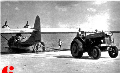
4 Next, the wheel units, consisting of two standard wheels and a regular Aerial strut are clamped into place on fittings provided for this purpose on the hull. These inspired the current amphibian version Consolidated Catalina.
